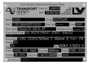
Vehicle inspectors shouldn't simply record the LVV certification plate number during a WoF inspection but should confirm that the vehicle matches the information recorded on the plate.
